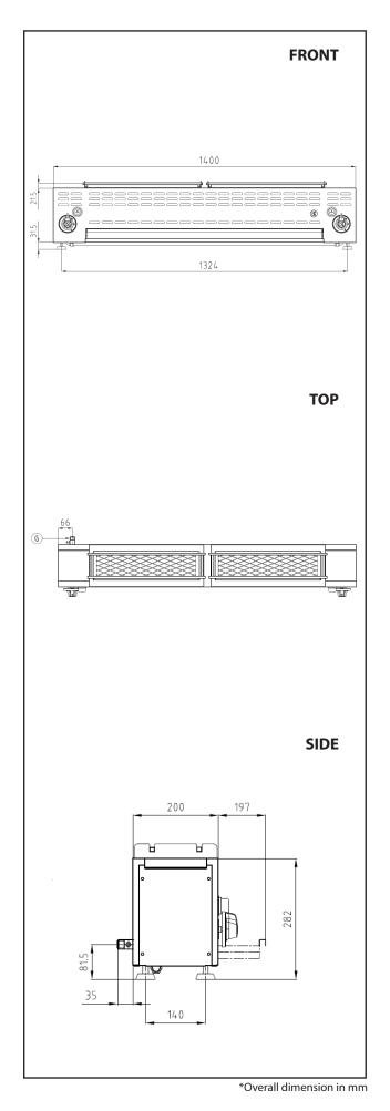
**TECHNICAL DATA External Dimensions** Width : 1400 mm : 200 mm Depth Height : 282 mm **Cooking Surface**
